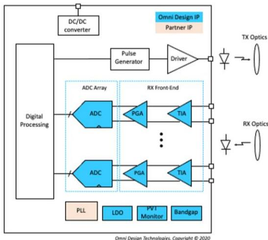
Pulsed-based LiDAR block diagram and available Omni Design IP
